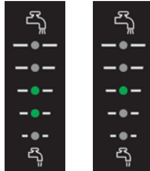
Fig. 14 SCALA2 outlet pressure indication
