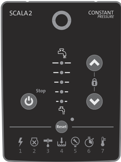
Fig. 13 SCALA2 operating panel
