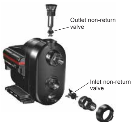
Fig. 20 Outlet and inlet non-return valves
